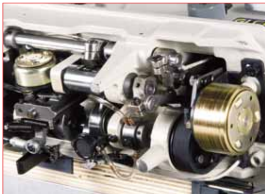
Solenoids for automatic trimming and back tack
