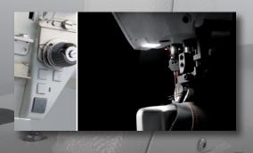
Easily adjustable thread trimmer with reinforced catcher and knife system for short thread ends (up to 15/3 syn.)
