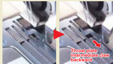
Throat plate intermediate claw forward/backward mechanism (for 2-needle machines)
